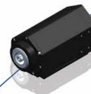
ES368 HSK E40/F50/F63 Power S1: from 6,5 to 11kW Torque S1: from 3,4 to 8,7Nm Max Speed: from 20000 to 36000rpm
